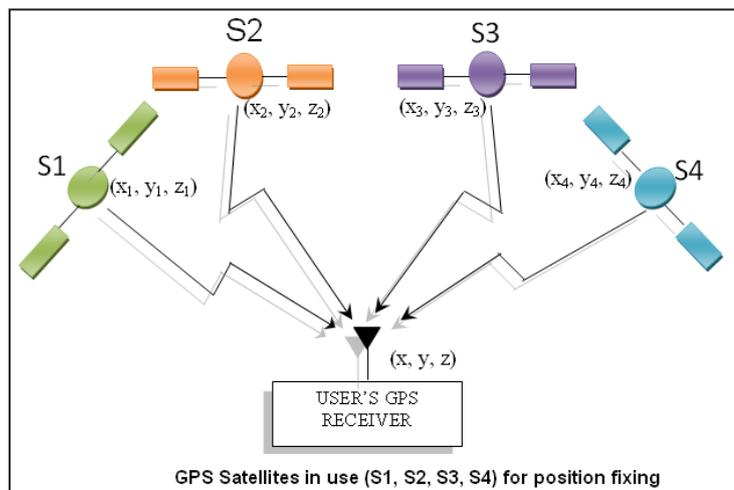
$10^8$  metres per second (299,792,458 m/sec to be more precise). This way the receiver calculates the range from the satellite, which is known as the pseudo range. This gives us a position circle on the surface of earth.
