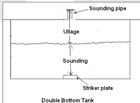
It is advisable to take soundings for ballast tanks and fresh water tanks, while for fuel oil tanks- it is generally advisable to take ullage readings. Ullage is the vertical distance between the surface of the liquid and the top of the ullage plug or the top of the sounding pipe. The following diagram describes the relationship between sounding and ullage
