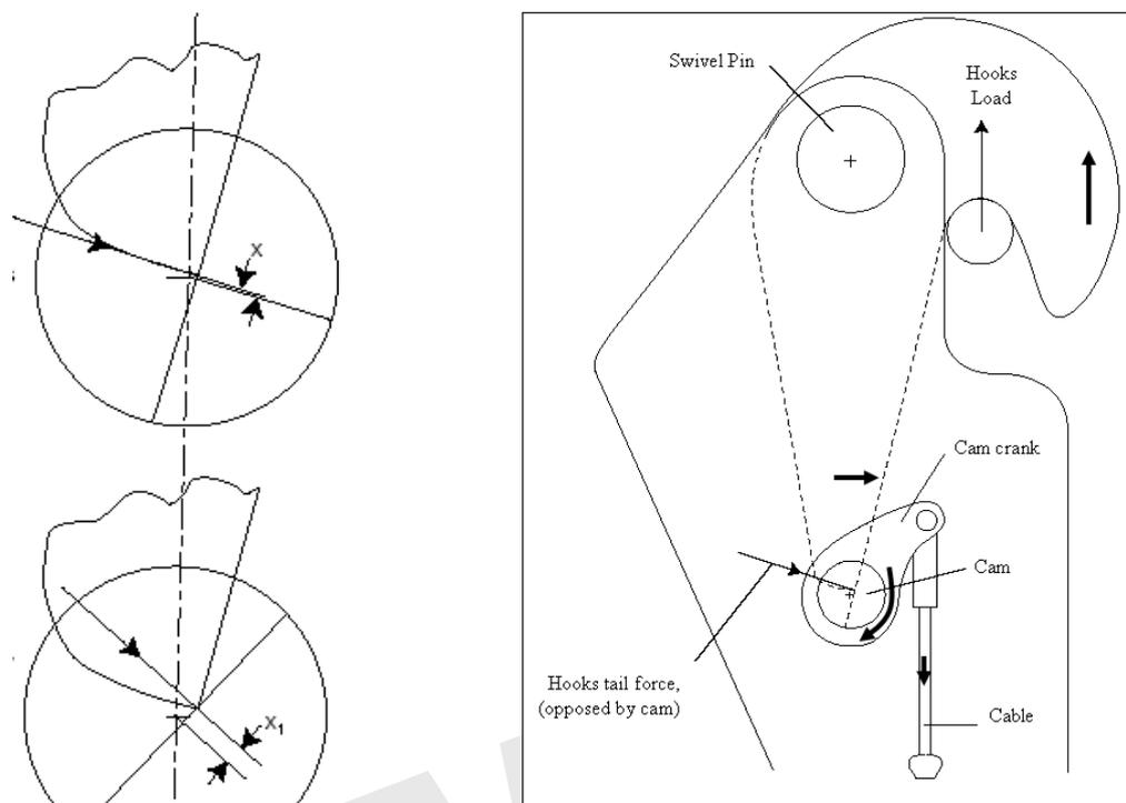
The diagram, showing the important features of resetting the mechanism, is complicated and makes it necessary to be able to clearly see the actual mechanism to understand its working.
