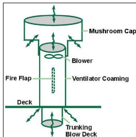
Flaps are provided below the blowers on the ventilator which can be closed to seal the entire compartment. The flaps will need to be closed in case of fire in the compartment or
