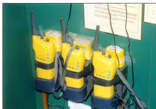
Along with the sets, primary sealed batteries are provided – these are to be used only in an emergency. In addition secondary type batteries are provided which can be charged. These batteries are used for trying out the sets. These sets must be tried out at least once a week.
