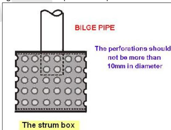
The suction pipe in each bilge has a filter at the end to avoid solid substances being carried away in to the pipe towards the pump. The filter is called a “strum box” and can be easily removed for cleaning. An open pipe without a “strum box” would result in clogging of the line and could also damage the pump. It must be in place during hold washing and before loading.
