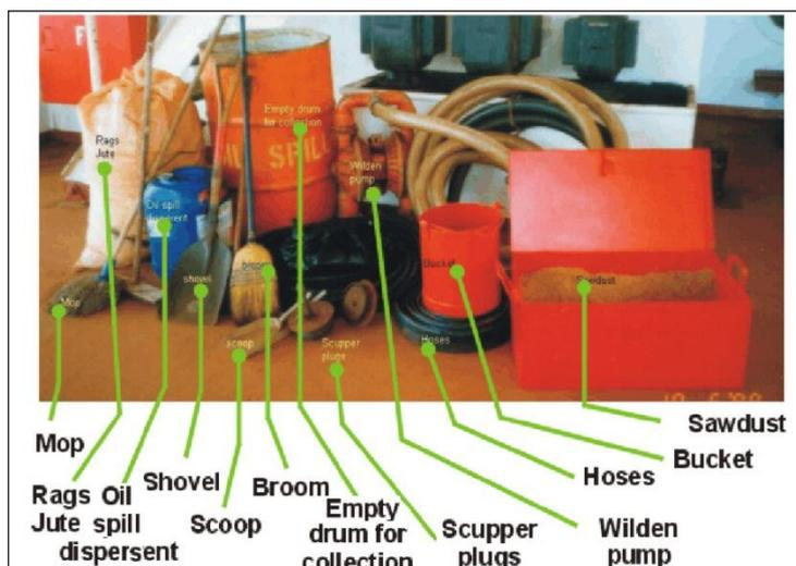
The following spill response equipment must be maintained on board.
