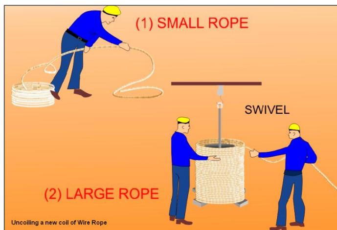
the shaft so that the drum is free to rotate. Then cut the straps and unreel the wire.
