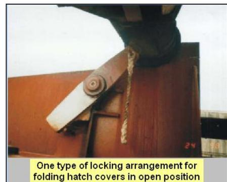
One type of locking arrangement for folding hatch covers in open position
