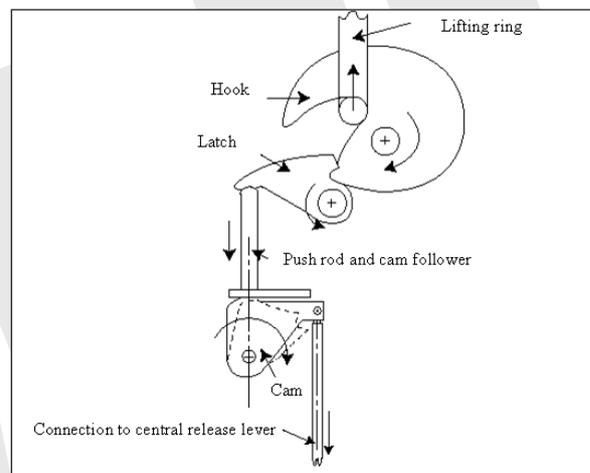
**Diagrammatic arrangement of hook release mechanism and the direction of movement of its components during release**
