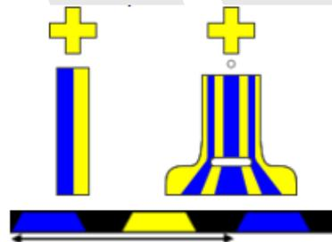
Figure 7: Emergency Wreck Marking Buoy
