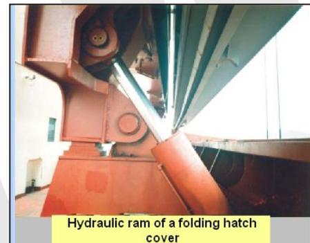
Hydraulic ram of a folding hatch cover
