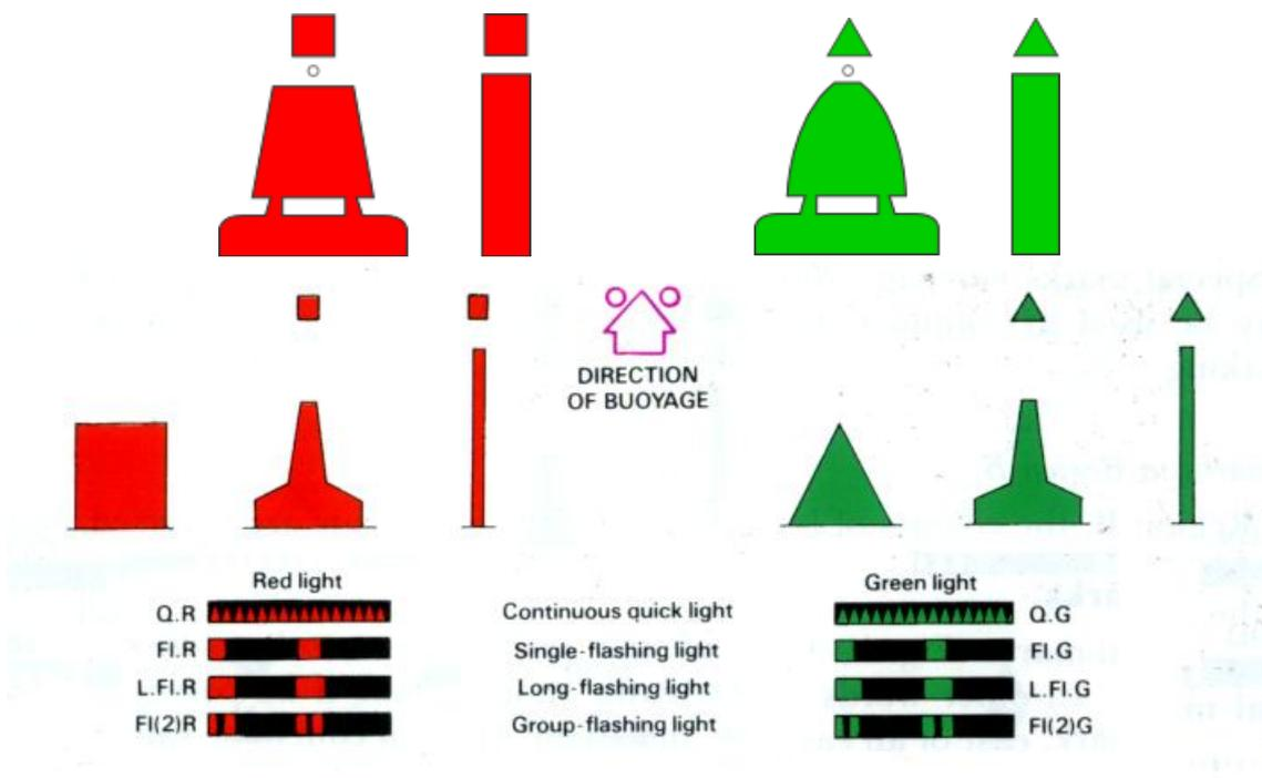
Figure 2a: IALA Region A: Port side buoys (Red), Starboard Side buoys (Green)
