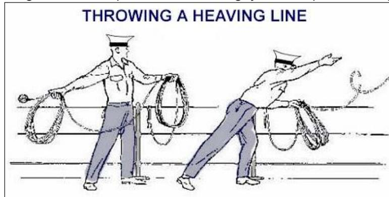
The heaving line should not be weighted by items such as shackles, bolts or nuts, or any other such objects; not attached directly to the heaving line and not inserted in the monkey's fist.
