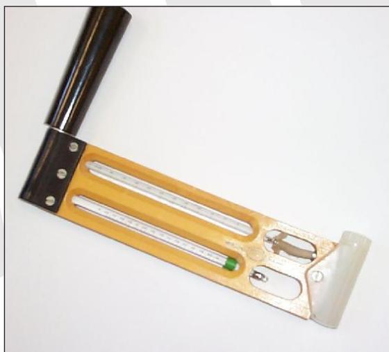
When a reading is to be taken, the wick is first wetted with water and then the instrument is whirled around. During the whirling, the water evaporates from the wick, cooling the wet-bulb thermometer. Then, the temperatures of both thermometers are read.
