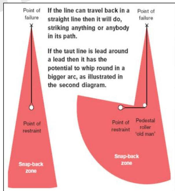
Snap back is common to all lines. Even long wires under tension can stretch enough to snap back with considerable energy. Synthetic ropes are more elastic therefore pose greater danger.
