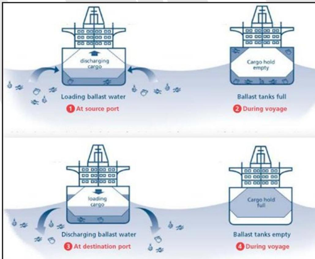
Ballast water is carried in unladen ships to provide stability. It is taken on board at the port while discharging the cargo, for stability purposes, before the voyage begins and tiny stowaways, in the form of marine organisms, are taken on board with it.
