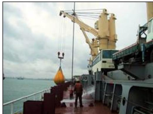
cranes. Some cranes have two SWL for different angles of jib clearly marked on the crane. Generally the reach in meters is marked.
