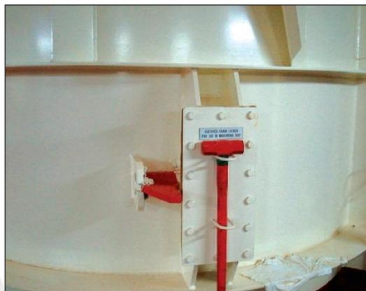
➤ In such cases the anchor chain is released from the bitter end. A quick release mechanism is provided for the purpose. Usually it comprises of a pin and hammer assembly whereby the locking pin for the bitter end is released by hammering it.
