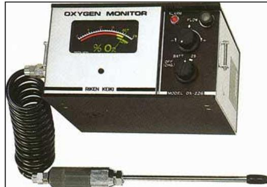
When testing is finished remove instrument from the test area and allows fresh air to be drawn into the instrument for at least 1 minute or until reading stabilizes at 21%. Always switch off the instrument after use and bring it back to its proper place of storage. Enter details of use in the usage log
