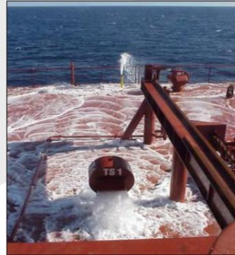
Ballast water is forced out an opening in flow-through exchange.
