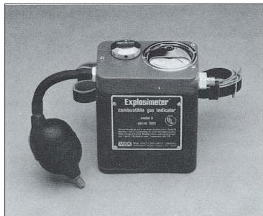
Explosimeter is device that is used to determine the content of hydrocarbon in the atmosphere. The scale used in the explosimeter is marked in terms of lower
