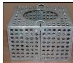
Strum boxes should be so constructed that they can be cleared without breaking any joint of the suction pipe.
