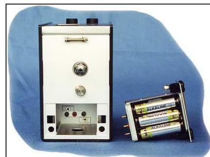
NOTE: The batteries should never be changed in a gas dangerous zone. Such instruments sometimes have dual scales each having a separate function. Attention to be paid to the scale in use.
