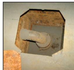
The bilge suction pipe ends in a strum box, which is also commonly known as 'rose box' situated in the inner compartment. The perforations in the strum box further help in filtering the liquid being sucked up and pumped out through the bilge pump.
