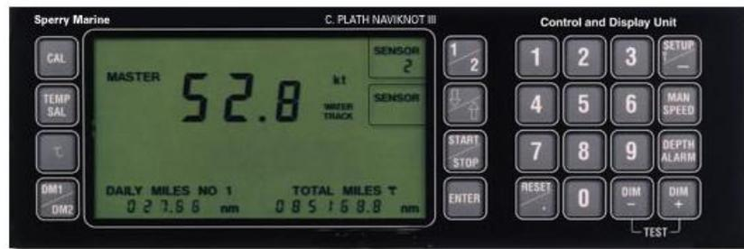
This type of log uses the Faraday-Maxwell induction law. This states that if a conductor cuts through a magnetic field, a small electro-magnetic force will be induced within itself which is proportional to the speed of the movement of conductor.
