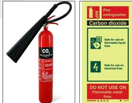
When handling the carbon dioxide extinguisher care must be taken to hold the hose only at the insulated handle provided for that purpose. If the extinguisher is held at the hose or at the discharging horn – the person is likely to get cold burns as the liquid carbon dioxide expands to gaseous state. Also, as intense cold is generated on discharge, the gas should not be directed on the exposed parts of the body.
