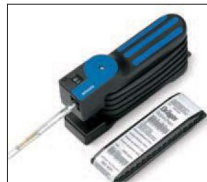
Toxic gas detection tube (e.g. draeger tube) is a vial which contains a chemical preparation that reacts with the measured substance by changing colour. To achieve the normal shelf life of 2 years the tube tips are fused at both ends. Thus, the vial provides an inert package for the reagent system. The printed scale allows a direct reading of the concentration. Thus, calibration by the user is not necessary.
