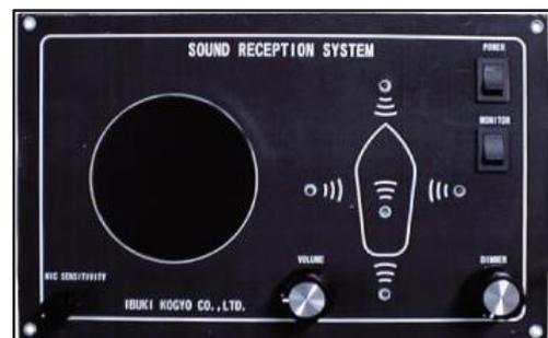
means of volume control. The volume control is capable of being set so that the sound pressure level of an incoming signal only is at least 10 dB (A) above the bridge noise level. Additionally the system has a display which gives a visual indication for at least 3 s of the incoming signals and their approximate direction.
