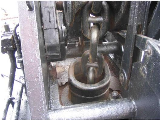
Spurling pipe capable of being closed watertight
