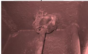
Hatch cleat in poor condition
