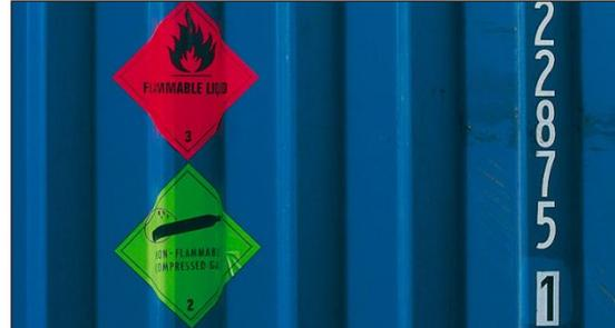
Placards minimum size 250 mm x 250 mm should be affixed to the exterior surfaces of the container to provide a warning that the contents of the unit are dangerous cargoes and present risks. These shall be so affixed as to be visible clearly.
