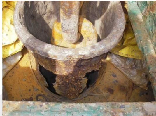
Badly corroded spurling pipe
