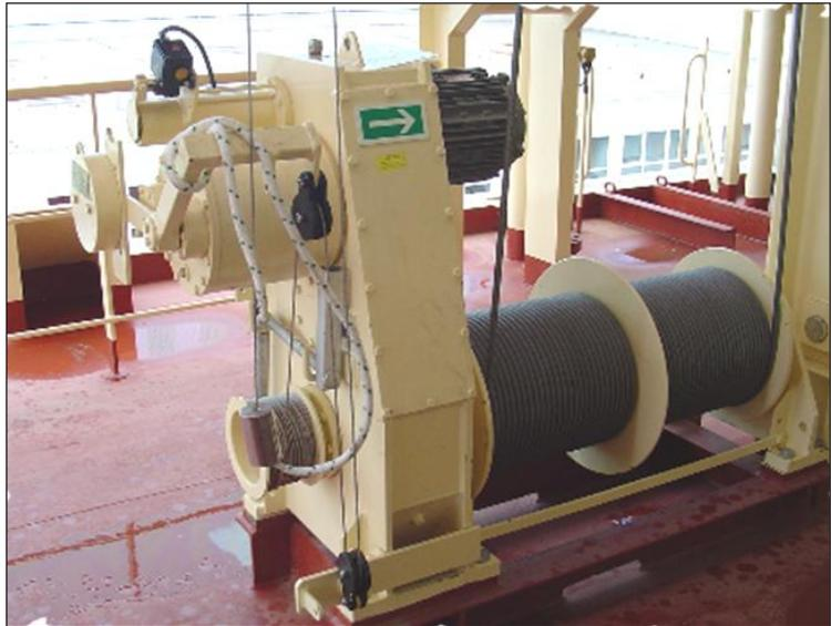
➤ The launching mechanism is so arranged that it may be actuated by one person from a position on the ship's deck and, except for secondary launching appliances for free-fall lifeboats, from a position within the survival craft or rescue boat. When launched by a person on the deck, the launching and recovery arrangements are such that the winch operator on the ship's deck is able to observe the craft at all times during launching and recovery.
